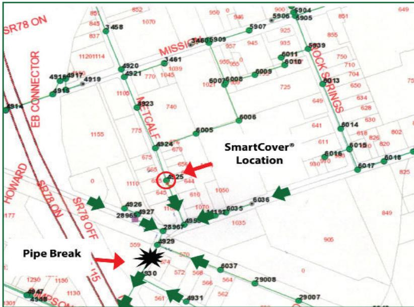
Inflow and Infiltration (I&I) is a high impact cost for utilities. It occurs when groundwater or storm water flows into the wastewater collection system, through cracked pipes, leaky manholes or unauthorized connections. Excessive I&I can overwhelm a collection system's capacity creating overflows. I&I also increases wastewater treatment plant flows unnecessarily driving up processing costs.
