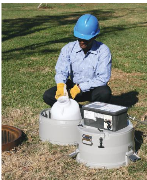
The 3700 sampler collects sequential or composite samples based on time or flow rate.
