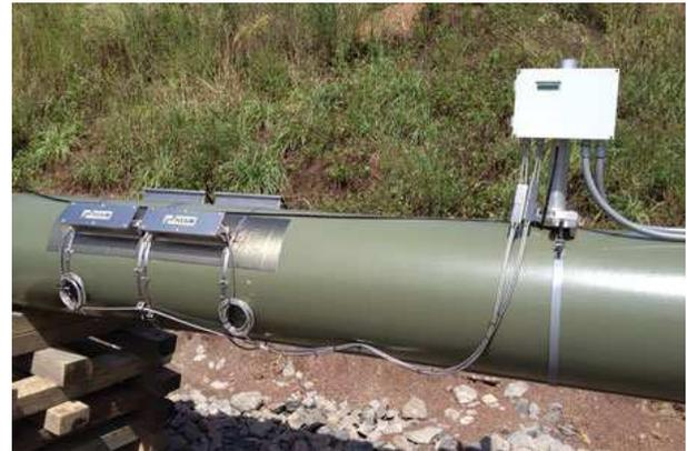
Ultrasonic flow meters clamp to the outside of the pipe, eliminating downtime while providing high accuracy.
