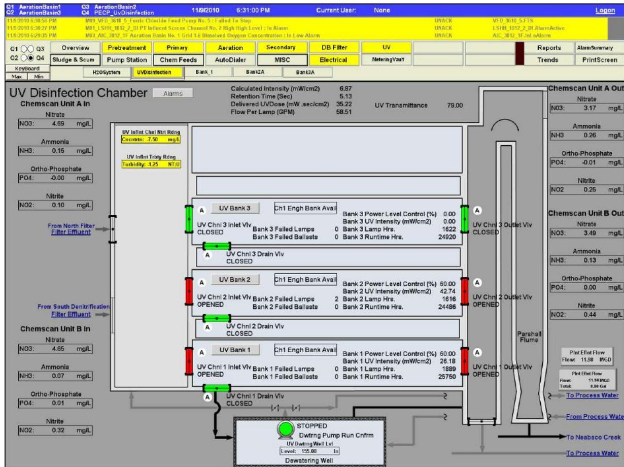
Figure 9 – Filters influent and effluent ChemScan units readings
