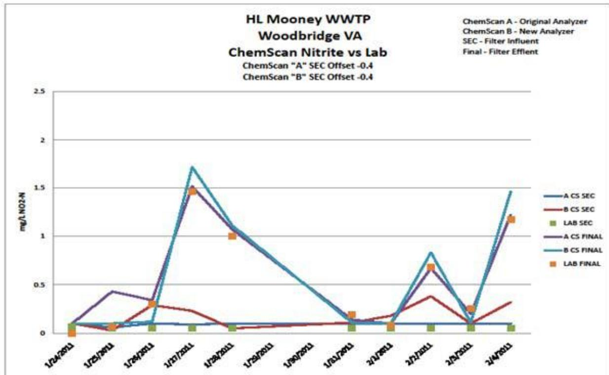
Figure 5 – ChemScan nitrite analysis during startup
