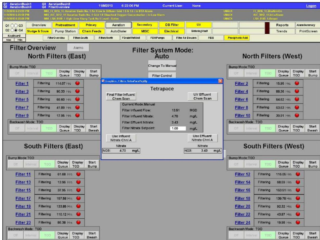
Figure 10 – Filters TETRAPace® calculation and ChemScan readings selection
