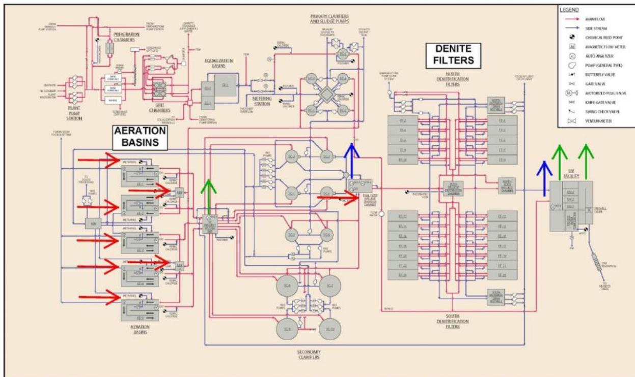
Figure 6 – Methanol application points and nutrient sample points
