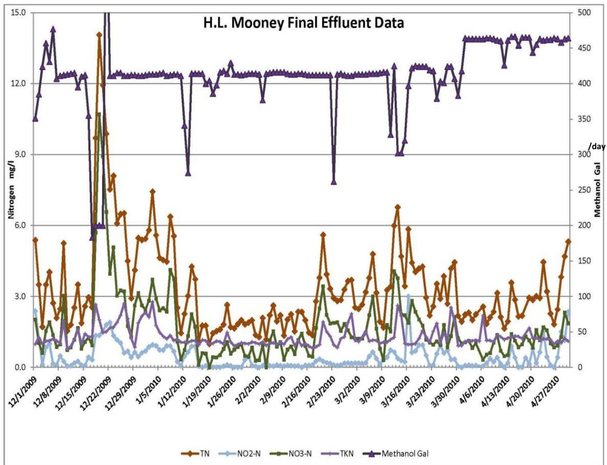
Figure 7 – Effluent nitrate and nitrite concentrations, and methanol feed rates *BEFORE* the upgrade
