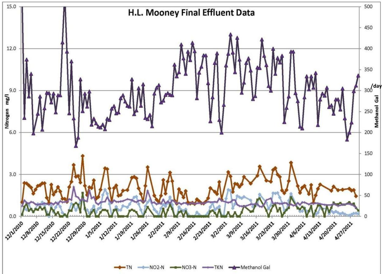
Figure 8 – Effluent nitrate and nitrite concentrations, and methanol feed rates *AFTER* the upgrade
