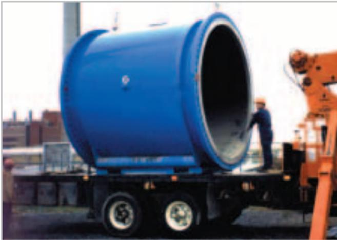
*Flanged version of the EMF primary head, ALTOFLUX DN 3000 mm, measuring range 0 ... 100.000 m<sup>3</sup>/h; 0 ... 400.000 USGPM*
