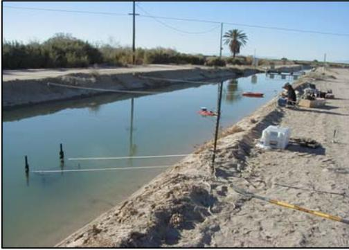
Figure 2 StreamPro ADCP attached to a pulley system 57 meters (187 feet) upstream Trifolium 13 Check structure; ChannelMaster H-ADCP mounted 7.6 meters (25 feet) upstream the pulley.
