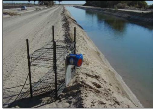
Figure 3 ChannelMaster H-ADCP prior to deployment.
