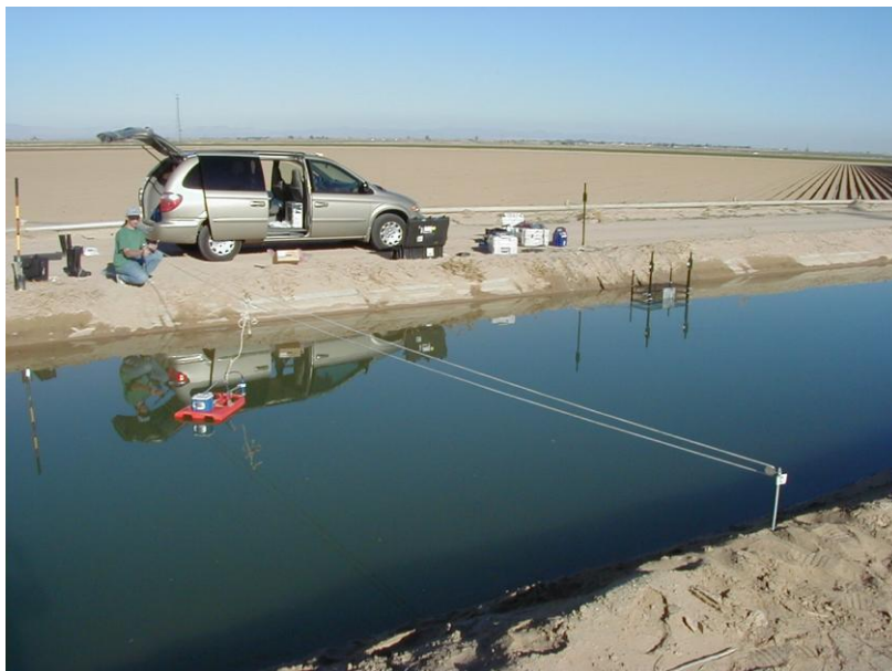
Figure 4 Field calibration test at an irrigation canal in the Imperial Irrigation District, California, using a StreamPro ADCP
